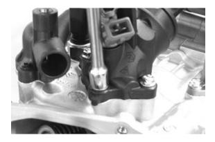
Loosen the three screws and remove the air intake manifold.
