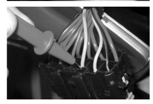
With the control unit and the injector disconnected, check the continuity of the Red-Yellow cable between pin 14 of the interface wiring and the injector connector
