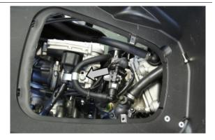
Remove the fast-release fitting from the injector support.
