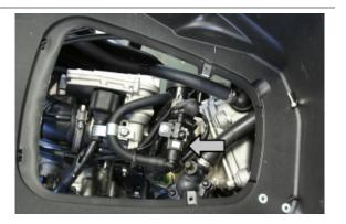
Check during regular operation by placing the appropriate tool between the pump and the injector. With the battery voltage> 12 V check that the fuel pressure is 2.5 BAR and that the input current is 1.4 to 1.8 A
