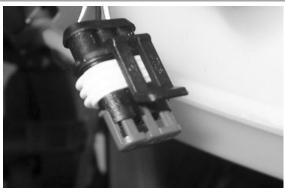
With the ignition key switch set to ON, check if there is battery voltage between the White-Black and Black cables.
