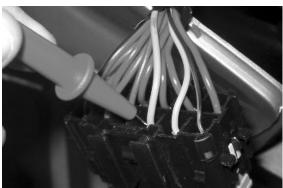
Check there is voltage between pins 22 and 26 of the interface wiring for around two seconds when switching to **«ON»**.
