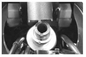
Insert the collar shown in the figure and restore the cable passage as shown in the figure.
