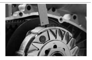
DO NOT OPEN THE MASSES USING TOOLS TO PREVENT A VARIATION IN THE RETURN SPRING LOAD.
