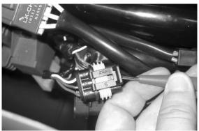
With the revolution sensor connector disconnected and interface wiring disconnected from the control unit, check that the red and white cables (pins 13 - 15) are isolated from each other and insulated from the ground connection.
