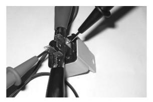
Check the power supply line of the injection load remote control energising coil: After switching to "ON", make sure there is battery voltage, for two seconds, between the black/white cable and black-violet cable of the remote control base. If there is not, check the continuity of the black/white cable between fuse block and the remote control base and of the black/violet cable between pin 20 of the control unit and the remote control base.
