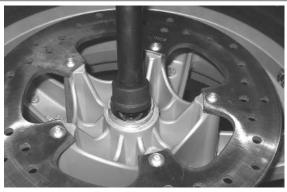
2 - Insert the two bearings one at a time using the punch consisting of adaptor handle, 32x35 mm adaptor and 15 mm guide, and take it to the stop.
