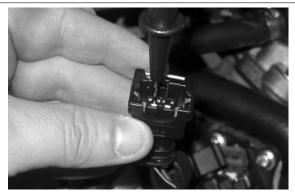
With injector disconnected and the injector load remote control disconnected, check the continuity of the Black-Green cable between the injector connector and remote control base.
