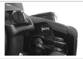
THE LEVEL TENDS TO DROP AS THE BRAKE PADS GET WORN, A MINIMUM LEVEL SHOULD NOT BE REACHED. IF THE LEVEL IS TOO LOW, CHECK AND FIX THE SYSTEM SEALS, IF REQUIRED. TOP UP THE PUMP TANK, IF REQUIRED, CONSIDERING THAT THE "MAX." LEVEL MUST ONLY BE OBTAINED WITH NEW PADS.
