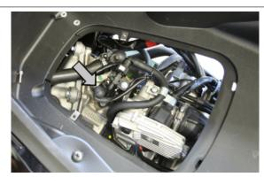
Remove the three screws fixing the manifold to the cylinder head and the clip fixing the throttle body to the manifold.
