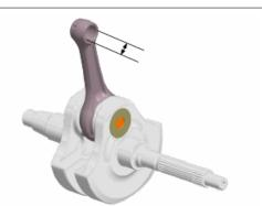
BUSHING INSIDE DIAMETER AFTER FITTING
