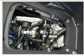
Remove the injector connector.
